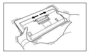
**5** Grasp the handle on the toner container and insert the toner container along the rail of the printer.
