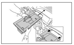
6 Hold the toner container by hands and fully insert it into the printer.
