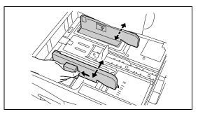
**3** Turn the paper stopper located at the right side of the paper cassette to the left as shown and move it to the desired paper size.
