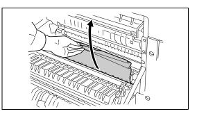
**3** Push the lever (green colored) to raise the duplex unit and remove the jammed paper.
